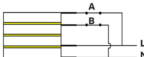
Alternative power output of the element when connected to a power supply:
